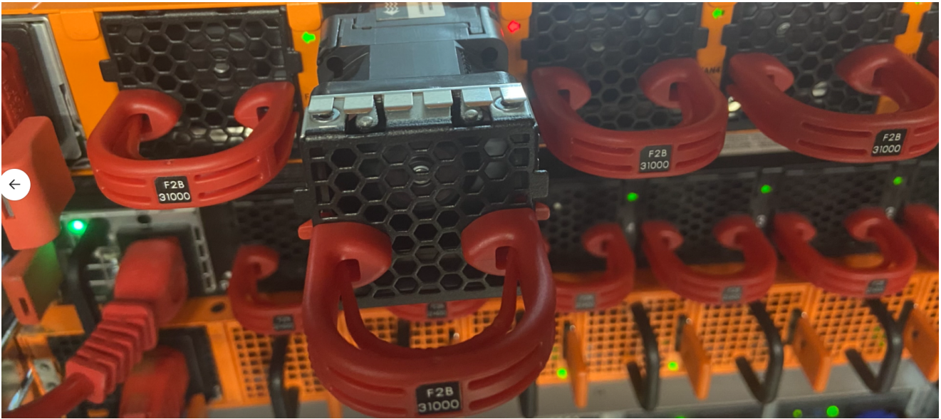
Figure 8 Replacing a Fan (GigaVUE-TA400E Shown)
